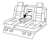
To gain access to the 60/40 load floor, store the cushion in the upright locked position. Pull up on the straps located at the sides of the load floor, and rotate forward until resting on the carpet.
